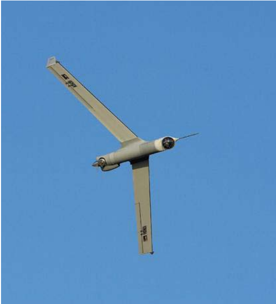
Insitu™ ScanEagle UAV Carrying an Altacam Vision™ Turret Photo courtesy Boeing
